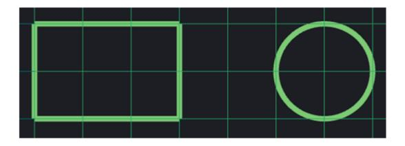
2. The slab entities are generated automatically in the enclosed areas formed
