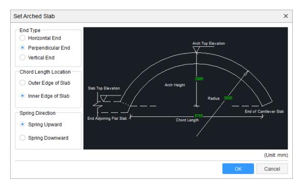
Perpendicular End and Inner Edge of Slab
